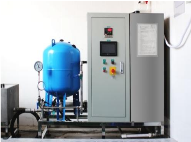
Water Hammer Test
